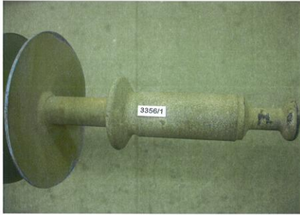
Figure (11): Appearance of insulator shank end fittings, both components are covered with fine dust and sand (Lab No. 3356/1).
