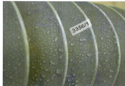
Figure (15): Lab.No. 3356/1 Hydrophobicity EC=1-2 in acc. with IEC 62073.
