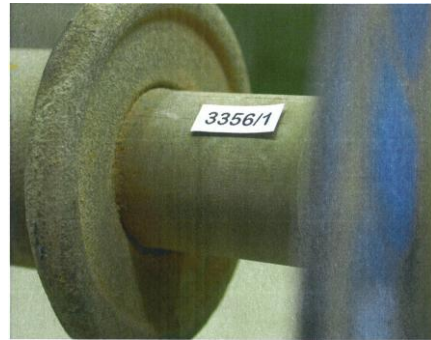
Figure (14): Lab.No. 3356/1 sealing area, sealing is full sound and intact.
