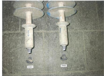
Figure (10): Lab. No. 3356/1-2: Mechanical failure modes after SML verification Test, UTS =181, 181kN, ball breakage, low scatter.
