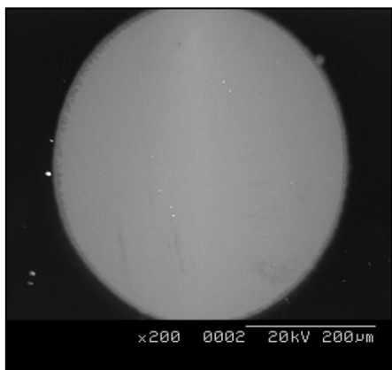
Figure 3: SEM photograph of 500 μm diameter Pt disk working electrode, at 200
