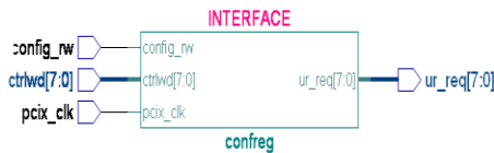
Fig 3 Interface of Configuration Register The Master Controller will receive the user request input and generates the control signals for Memory or IO read/write operations, receive/transmit mode, target retry and disconnect signals shown in fig4.
